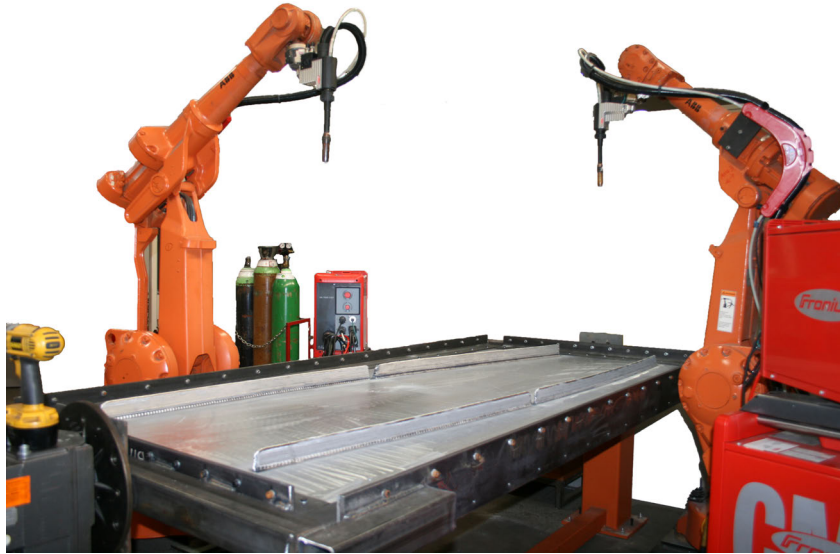
Figure 3: 2.5 m long aluminium rib. For this component, WAAM has enabled material savings of more than 500 kg.
